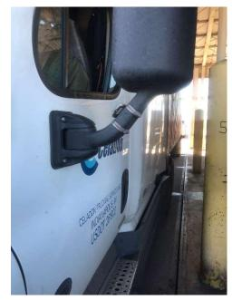
To ensure the highest degree of RFID read accuracy, it is expected that the RFID tag is mounted on the mirror bracket.
